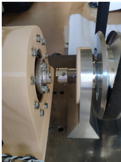
Fig. 2.9. The damaged torque transmission part
